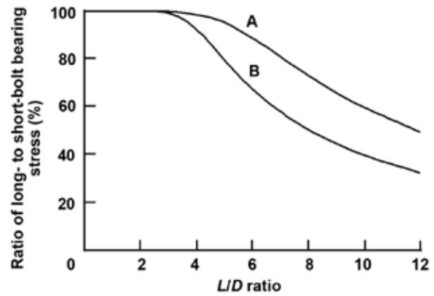
Figure 8–12. Variation in the proportional limit bolt-bearing stress parallel to grain with  $L/D$  ratio. Curve A, bolts with yield stress of 861.84 MPa (125,000 lb in<sup>-2</sup>); curve B, bolts with yield stress of 310.26 MPa (45,000 lb in<sup>-2</sup>).
