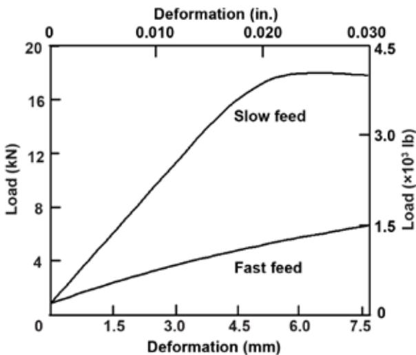
**Figure 8-15.** Typical load–deformation curves showing the effect of surface condition of bolt holes, resulting from a slow feed rate and a fast feed rate, on the deformation in a joint when subjected to loading under bolts. The surface conditions of the bolt holes were similar to those illustrated in Figure 8-14.
