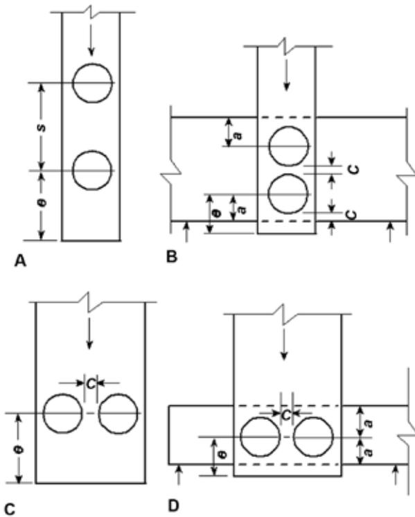
**Figure 8–25. Types of multiple-connector joints:** A, joint strength depends on end distance  $e$  and connector spacing  $s$ ; B, joint strength depends on  $e$ , clear  $c$ , and edge  $a$  distances; C, joint strength depends on end  $e$  and clear  $c$  distances; D, joint strength depends on end  $e$ , clear  $c$ , and edge  $a$  distances.
