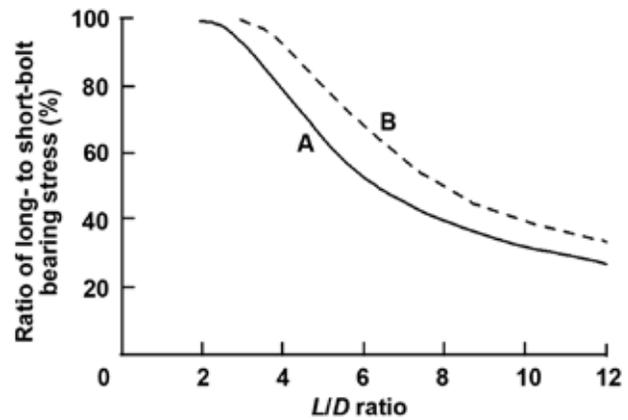
**Figure 8–9. Variation in bolt-bearing stress at the proportional limit parallel to grain with  $L/D$  ratio. Curve A, relation obtained from experimental evaluation; curve B, modified relation used for establishing design loads.**
